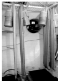
Figure 5: Battelle curtains deployed during early USN trial using LiOH canisters. Each curtain is approximately 6 feet long.
