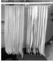
Figure 4: Reactive Plastic Curtain cut to length and hung in strips during a USN trial.
