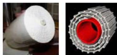
Figure 3: Picture of RPC removed from storage canister; diagram of a section of RPC sheet, ribbed for tuned air flow.
